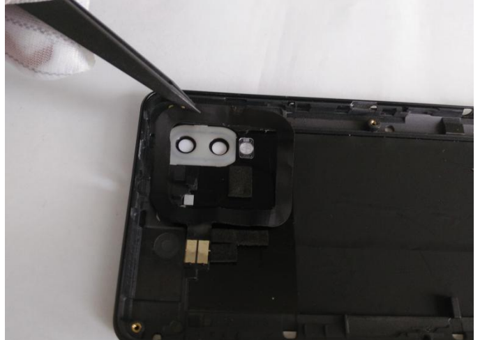
64、Dismantling NFC antenna by plastic tweezer.
