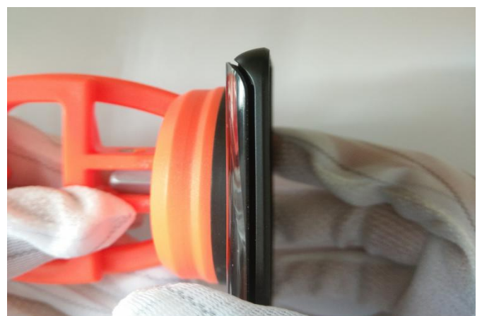
78、Sucking the middle part of the phone screen by suction cup(the middle part of a curved screen is flat), holding the border in the other hand and splitting it apart. (NOTE: do not PULL, seperating it with even force. During the separation process, it can be heated simultaneously.
