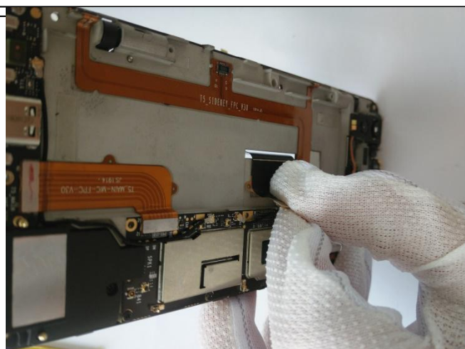
22、Tearing off FPC by hand after heating it by hot air gun (80°C)
