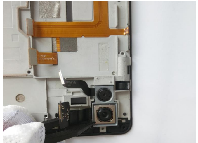
46、Dismantling camera assembly by plastic tweezer.
