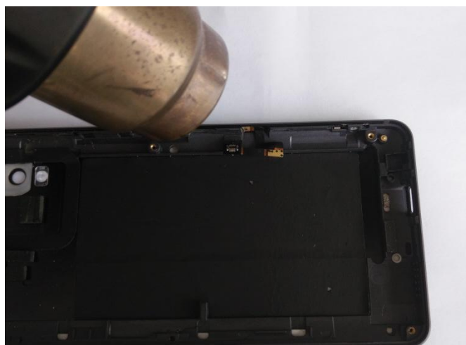
60、Heating fingerprint FPC by hot air gun at 80 degree.
