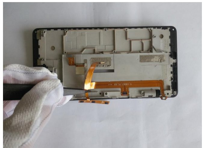
48、Dismantling side FPC by plastic tweezer.
