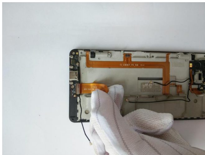
32、 After heating the main FPC for a while by hot air gun at 80 dreg ree, then dismantling it.
