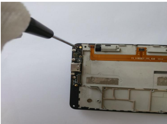
41、Opening the screws of USB board by screwdriver.
