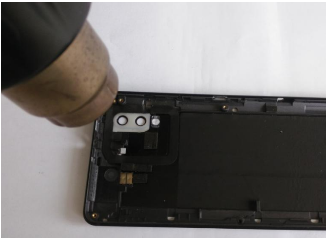
63、Evenly heating NFC antenna area by Hot air gun at 80 degree.
