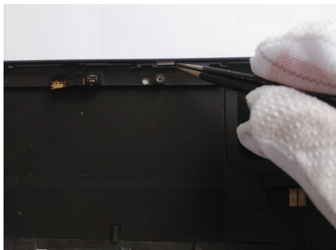
56、Peeling off the steel disc by inserting the tweezer into the gap between the side key
