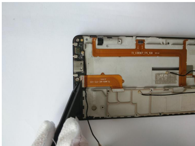
31、 Seperating main FPC connector of USB board by plastic tweezer.
