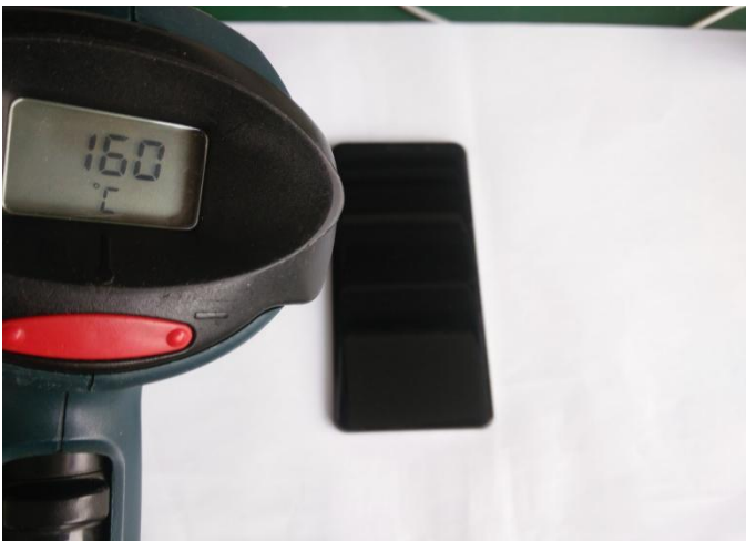
75、Adjusting the hot air gun at 160 degree.(note: Heating platform doesn't apply to curved screen.)
