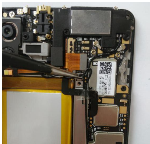
17、Sorting out the coaxial line of sheet steal by tweezer.
