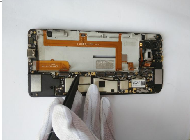
24、Separating button placement of coaxial line of main board by plastic tweezer.
