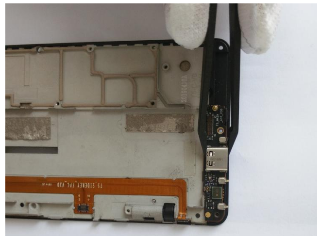
42、Dismantling USB board by plastic tweezers.
