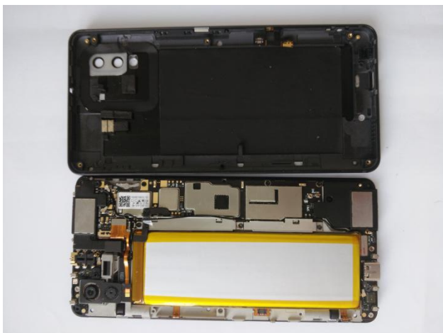
15、Dismantling the bottom cover.
