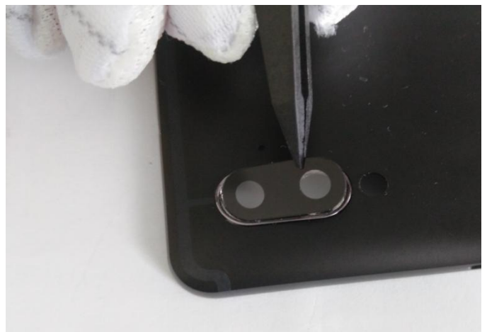
62. Pushing the camera slice from inside out by plastic tweezer and dismantling the back camera
