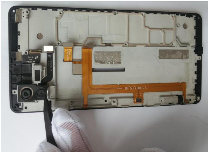
45、Peeling the foam of camera by plastic tweezer
