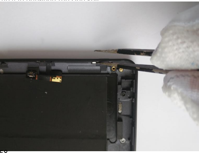
58、Peeling the steel disc by inserting the tweezer into the gap between camera button.
