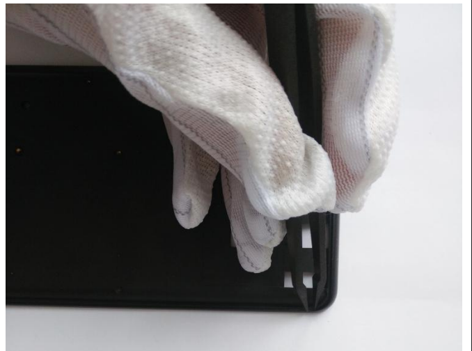
82、Cleaning residual gel along the edges by plastic tweezer.
