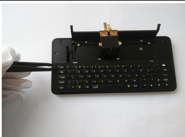
11、After 5-6 mins heating, dismantling the keyboard along its edges by plastic tweezer.
