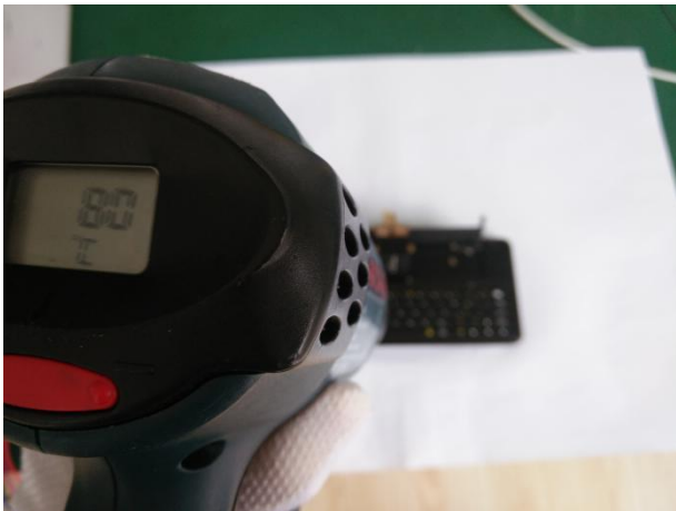
9、Adjusting the temperature of hot air gun to 80°C.
