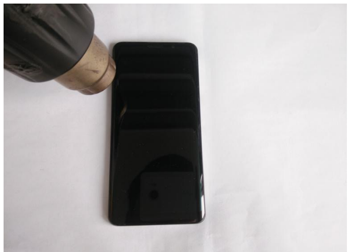
76、Evenly heating the four edges along the screen by hot air gun.
