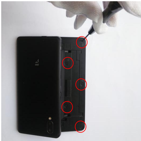
3、Opening five screws of the bottom base(Shown
