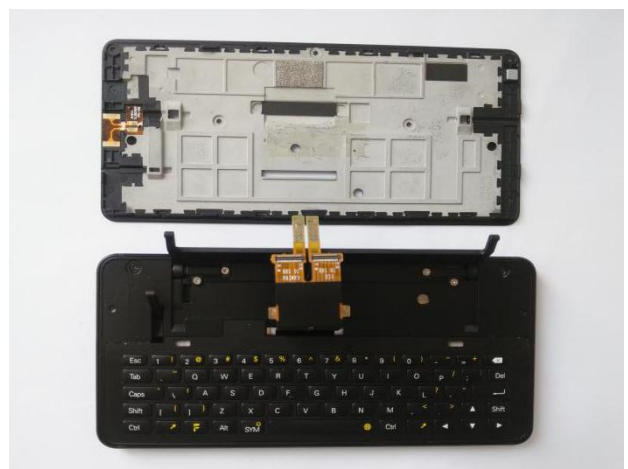
8、Dismantling bottom base( Mind FPC cable of screen)
