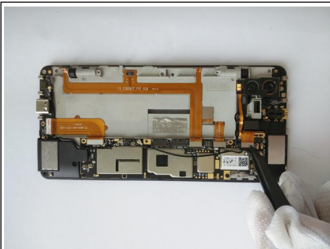
23、Dismantling flash light, front& back camera, keyboard, side buttons, main FPC and other connector in sequence by plastic tweezers. (Mind surrounding components.)
