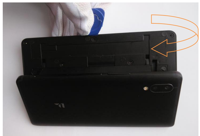
4、Inserting the chip in the gap between the cover and bottom case, rip the cover along edges.
