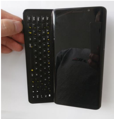
1、Power off and push the keyboard, getting the tray out.
